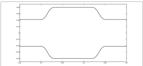
**Fig. 6** Precatalyzer with connections made by double parabolae (the next case with connections made by cubic arcs looks very similar)
