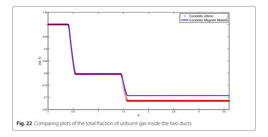
When two catalyzers have different volumes but yield similar results, it happens precisely this: the catalyzer with a larger radius, in order to provide the same result as the other (with a smaller radius), requires a higher exposition of the gas to the reacting substances, hence to be longer.
