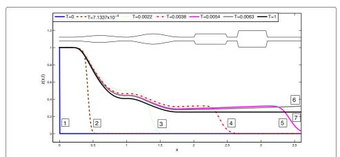
**Fig. 15** Case (h): Time evolution of unburnt gas using *two cosinusoidal arcs*. Solutions are numbered according to time: the blue curve is the initial state, the black curve is the final one, at time T = 1; z(L, T) is the fraction of unburnt gas injected into the atmosphere
