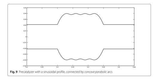
Starting from the typical Magneti Marelli's device, where the various pieces are schematically connected as in Fig. 3, we first modify the joints, choosing for them linear, parabolic or cubic arcs, double parabolic arcs, and sinusoidal profiles. Finally, we will change completely the original shape of the catalyzer.
