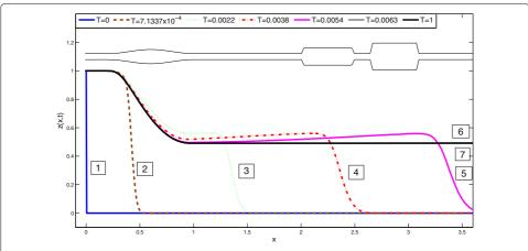
**Fig. 17** Case (i): Time evolution of the fraction of unburnt gas using *a cosinusoidal arc*. Solutions are numbered according to time: the blue curve is the initial state, the black one is the final one, at time T=1; z(L,T) is the fraction of unburnt gas injected into the atmosphere
