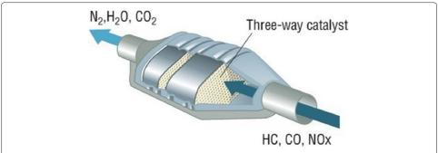
**Fig. 2** A three-way catalytic converter. Note the honeycomb structure. (By courtesy of AA1Car; reprinted with permission)
