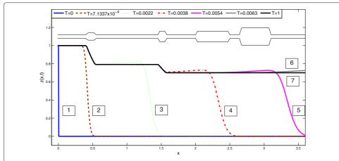
**Fig. 14** Case of profile in (a): Time evolution of the total fraction of unburnt gas, z(x,t), when *linear joints* between the various components are used. Curves are numbered according to various times: the blue line is the initial state, the black line the solution at the final time, T = 1. At the end of the duct, x = L, the value of the fraction of unburnt gas, z(L, T), injected into the atmosphere can be read
