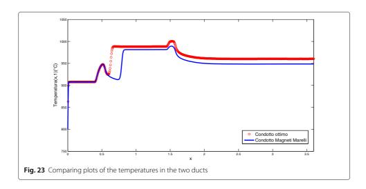
Similar considerations can be made for the catalyzer. The best result we obtained was that with  $L=0.07\,m$  and  $r_2=0.04\,m$  (see Table 5). Using these two devices together, a fraction of unburnt gas at the duct's end about equal to 0.6859 was obtained, while for the Magneti Marelli device we have 0.7075. In Fig. 22, these two cases are compared, and on Fig. 23, the temperatures are compared.
