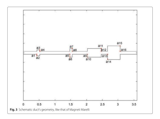
$$\begin{cases} \rho(x,0) = 1.21 \, Kg/m^3; & \rho(0,t) = 1 \, Kg/m^3; \\ u(x,0) = 413.22 \, m/s; & u(0,t) = 600 \, m/s; \\ \theta(x,0) = 295 \, ^{o}C; & \theta(0,t) = 800 \, ^{o}C; \\ p(x,0) = 1.0247 \times 10^5 \, Pa; & p(0,t) = 2.2966 \times 10^5 \, Pa; \\ z(x,0) = 0; & z(0,t) = 1. \end{cases}$$
